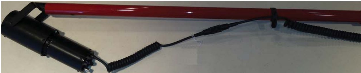
Picture 1: Fasten the axial cable lead to the pole using the rubber strap provided.
